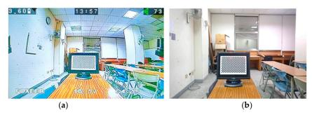
**Figure 3.** Camera's field of view and lens distortion. (a) original UAV camera image (b) inspection camera image.
