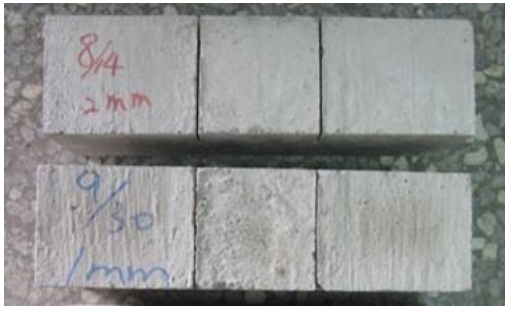
Fig. 1 Superficial cracks on the test samples with 1-mm width (lower) and 2-mm width (upper)
