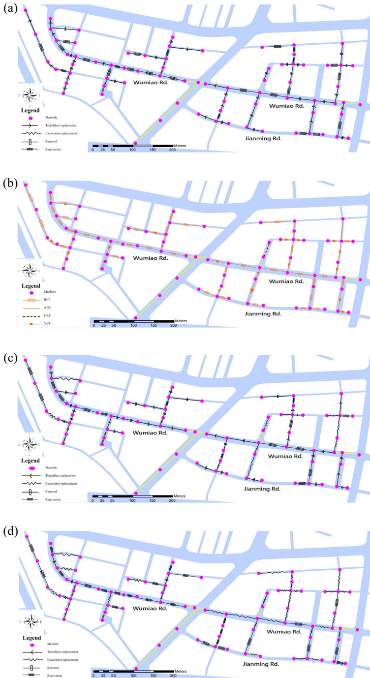
Fig. 7 Layout of a rehabilitation method and b substitution material in maximum pipe service life plan. Layout of rehabilitation methods in c minimum traffic disruption plan and d minimum rehabilitation cost plan
