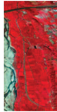
Fig. 3. Raw ISIS images in 1.16m ground resolution (2250 lines x 1150 pixels; Red: \lambda_{182}=869.9\text{nm} , Green: \lambda_{94}=654.6\text{nm} , Blue: \lambda_{52}=551.9\text{nm} ).
