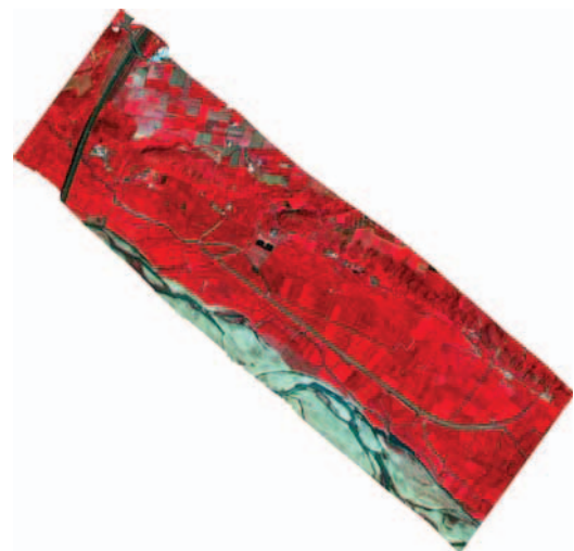
Fig. 4. Self-calibrated DG rectified ISIS images in 1.0m ground resolution (2998 lines x 3133 pixels).
