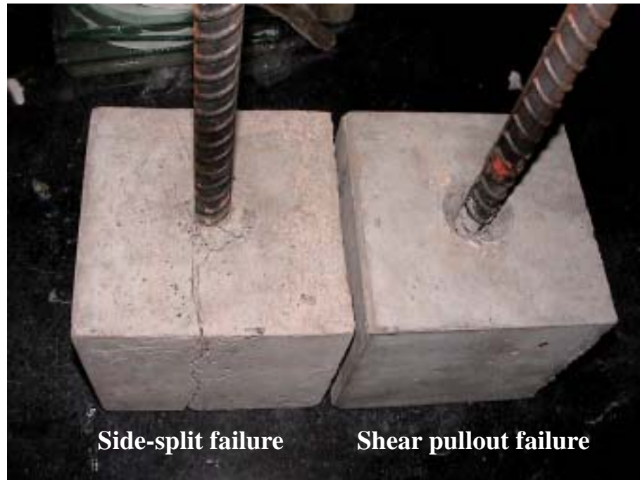
Figure 5 Comparisons of the failed specimens
