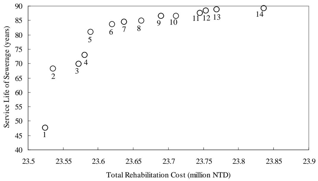
Fig. 7. Optimal Pareto curve of sewer rehabilitation
